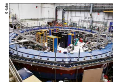
Left: the centrepiece of the Fermilab g-2 experiment (E989) is a 14-m-diameter electromagnet that generates an ultra-uniform magnetic field. Right: a typical anomalous-precession-frequency plot made from higher-energy positrons vs time-in-fill of muons in the storage ring. The 60-hour sample, when fitted (green) to a functional form that includes beam dynamics, pileup correction and basic gain stabilisation, gives a good \chi^2 and a statistical precision of about 1.2 ppm.
