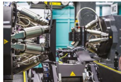
Image 3: Hexapods align the X-ray optics in up to six axes. Additional goniometers allow rotation around the beam path. (Source: PI)
