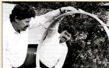
An inflatable mirror made from an aluminised mylar membrane 25 µm thick, which has been developed at the CERN West Workshop. By varying the pressure applied to the membrane the mirror takes up varying quasi-spherical forms. The focal length can thus be varied for use in a Cherenkov counter.
