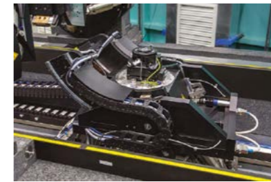
Image 4: The positioning mechanics of the sample module: the hexapod with its six active and six redundant struts for position feedback sits underneath. The goniometer guides are above and alignment in the X, Y, and Z direction as well as the rotation stage setting are visible. (Source: PI)
