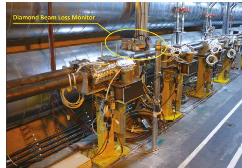
The CIVIDEC Diamond Beam Loss Monitor at the LHC collimation area IP7.
