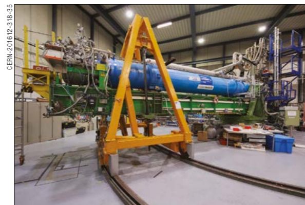
Fig. 5. The CAST experiment at CERN, which reuses a prototype dipole magnet from the LHC, photographed in December 2016.
