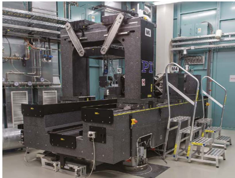
Image 2: The massive granite construction of the base guarantees the necessary overall stiffness of the system. Hoverpads allow easy moving of the 20-ton machine. (Source: PI)
