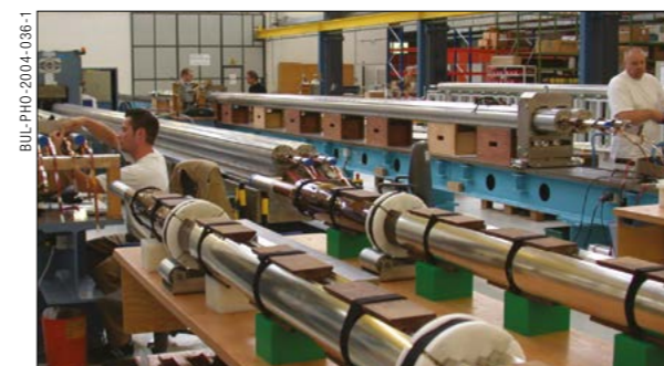
Fig. 2. The main components and tooling required to assemble the LHC dipole cold-masses were purchased by CERN and delivered to contractors (left, showing cold masses at German company Noell in 2003), who would then return the assembled cold masses to CERN for final insertion into the vacuum vessels (right, showing the final dipole being lowered into the LHC tunnel in April 2007). This approach was also applied to the superconducting strands and cables, the quantities of which were so huge that all major European manufacturers, as well as one US and one Japanese firm, were involved.
